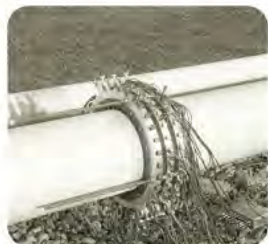
Transducer ring, early site test (circa 1994)
