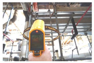
A temperature reading of 242°C (468°F) on the surface of the 8" diesel line.
