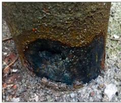
**Indication A1.** A through-wall defect located on the section just above the ground interface of the lamp post.
